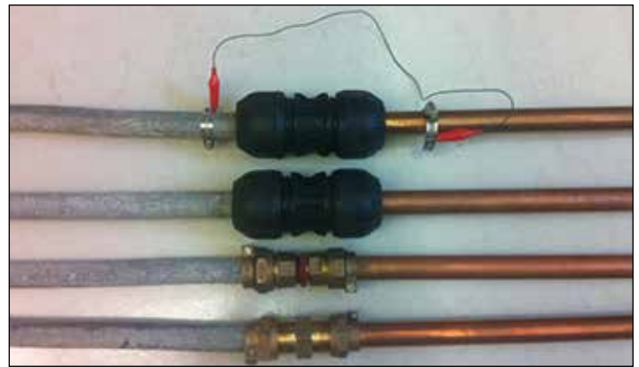
During this research four couplings were used to connect lead pipe and copper tubing.
